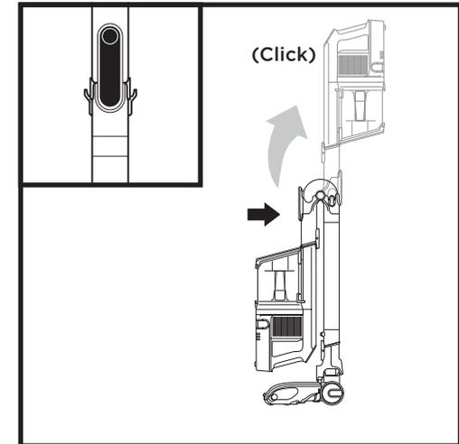
To take the vacuum out of storage mode, press the unlock latch and lift up the handheld vacuum until the wand clicks and locks into place.
