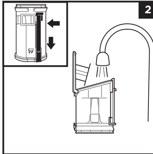
To clean the interior of the dust cup, rinse it with water. Place it on its side with the lid open to air-dry for at least 24 hours before reinstalling.
