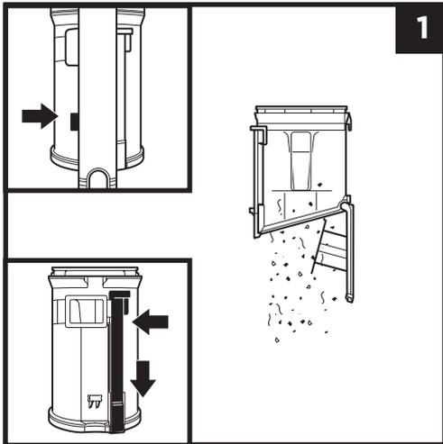
To remove the dust cup from the handheld vacuum, press the **Dust Cup Release** button near the handheld vacuum nozzle. Tilt the dust cup and lift off to remove.
