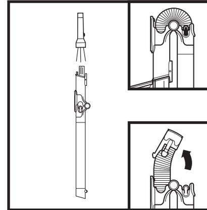
Checking for Blockages in the Floor Nozzle:
