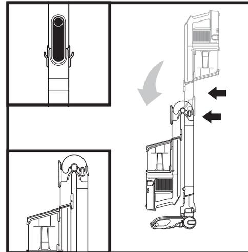
To put the vacuum in storage mode, press the unlock latch while folding the handheld vacuum forward.
