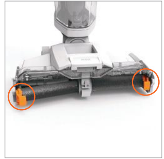
Lift and pull the tab on the outer side of each brushroll and pull to remove.
