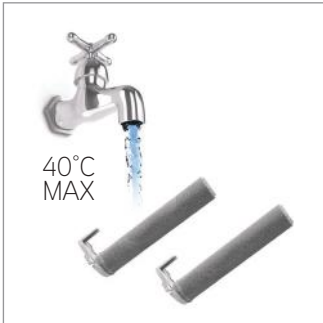
Rinse the brushrolls and brushroll cover in water (40°C max). Allow brushrolls to dry in tray storage before refitting.
