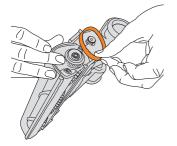
Replace the old belt, ensuring the teeth are fully engaged with the cogs.
