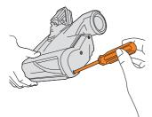
Using a crosshead screwdriver, remove 3 screws from the side of the floor head.
