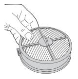
Check the post-motor filter for discolouration.
