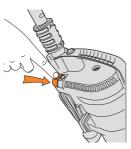
Plug in your machine and push ON/OFF button to switch on.
