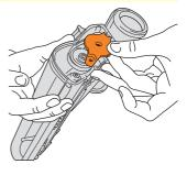
Remove the brush bar location plate to gain access to the belt.
