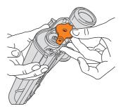
Remove the brush bar location plate to gain access to the belt.
