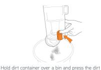
container release button to open allowing dirt to fall out.
