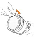
Grasp tab on filter and pull to remove.
