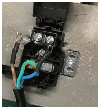
Fasten the wires beneath the screw heads
