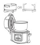
2 Follow the steps above to install the pressure lid on page 16. Turn the pressure release valve to the VENT position.
