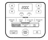
2 Use the up and down TIME arrows to set the cook time in minute increments up to 1 hour.
