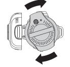
**3** Make sure the pressure release valve on the lid is in the SEAL position.
