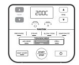
2 Use the up and down TIME arrows to set the cook time in minute increments up to 1 hour, 5-minute increments from 1 hour to 4 hours.
