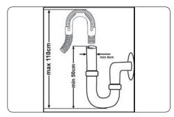
Connect water drain hose directly to water drain hole or to the sink outlet spigot. This connection should be minimum 50 cm and maximum 110 cm from floor plane
