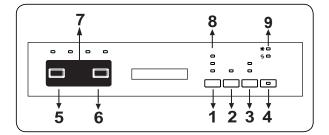
You can press the On/Off button (4) to switch on the product. On/off lights will be on so long as the machine is on. Press the program button (5) to set the suitable program.
