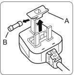
The mains lead of this appliance has been fitted with a BS 1363A 13A fused plug. To change a fuse in this type of plug, follow the steps below:
