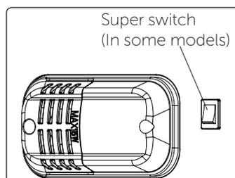
**Winter Switch:** If ambient temperature is below 16 °C, this switch shall be used as winter switch and it keeps your fridge above 0 °C while freezer is below -18 °C in low ambients.
