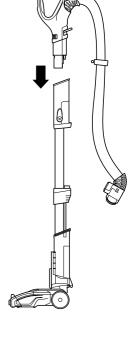
1 Place motorised floor nozzle on floor and insert wand.
