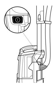
2 The Powered Lift-Away DuoClean has a 2-speed Slider Switch on the handle. Move the Slider Switch to appropriate speed setting. The soft roller spins in both settings to pick up extra dust and debris.
