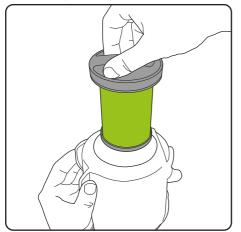
Remove the filter by pulling it from the top of the bin. Tap the dirt from the filter and tip any dirt from the filter housing. Wash the filter if necessary.
