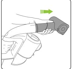
Gently pull the Power Brush from the Multi to remove. The battery should be removed when changing attachments.
