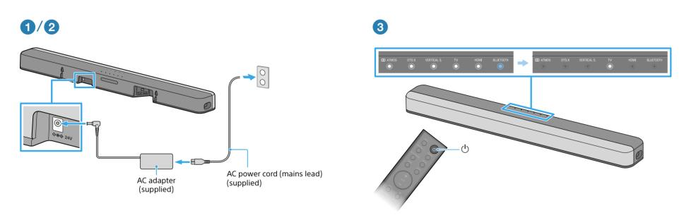
1 Connect the AC power cord (mains lead) (supplied) and the AC adapter (supplied), and then insert the plug of the AC adapter into the DC IN terminal of the Sound Bar until it clicks.
