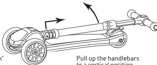
Pull up the handlebars to a vertical position.
