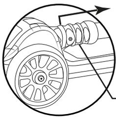
Pull the 'handlebar lock' to release.
