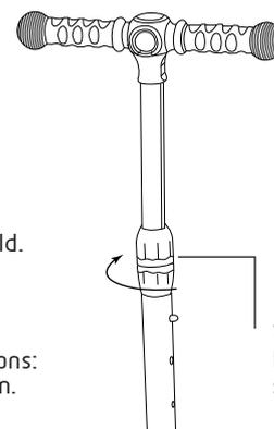
When at the desired height, screw tight the stem adjuster.
