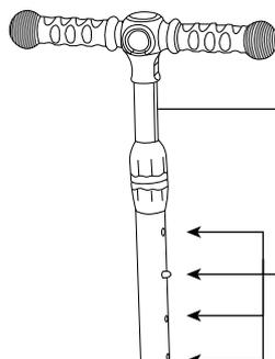
Push in the button and pull the handlebars up and down until it is the correct height for your child.
