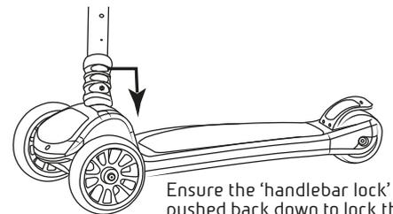
Ensure the 'handlebar lock' is pushed back down to lock the bars in position.
