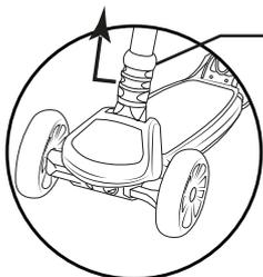
Pull up the 'handlebar lock' to release.
