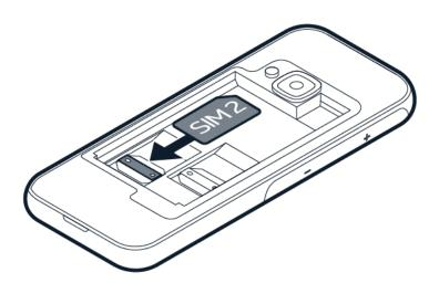
If you have a dual-SIM phone, slide the second SIM in the SIM2 slot. Both SIM cards are available at the same time if neither of them is being used, but while one SIM card is active, for example, making a call, the other may be unavailable.
