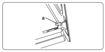
**3.** Close the door until it almost reaches the fully closed position and remove the door by pulling it towards you.
