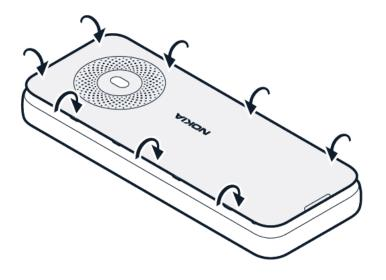
Put back the back cover and press around the edges until the cover snaps into place.
