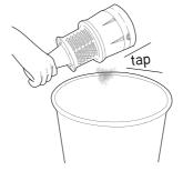
Tap over a bin to remove dirt and debris.
