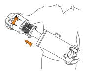
Lift to remove the separator from the dirt container
