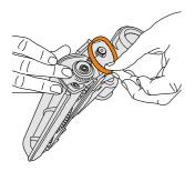
Clean any debris from the cogs. To replace the belt firstly hook the belt over the small cog. Slide the belt over the top of the large cog and rotate the belt and cog anticlockwise. During rotation the grooved belt will slide onto the cog.
