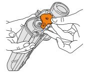
Pull to remove the brushbar location plate. Remove belt.
