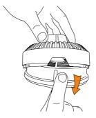
Remove the post-motor filter from the filter cover.
