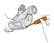
Using a crosshead screwdriver, remove the 3 screws from the belt cover on the side of the floorhead.
