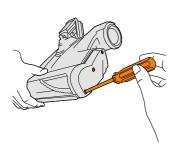
Using a crosshead screwdriver, remove 3 screws from the side of the floorhead
