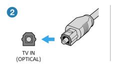
When there is no HDMI IN jack labeled "ARC" on your TV, use the optical digital cable (supplied) to connect an optical out jack on your TV and the TV IN (OPTICAL) jack on the Bar Speaker.
