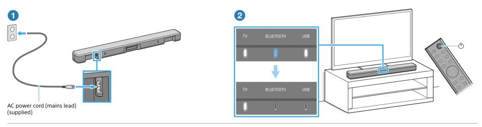
**1** Connect the AC power cord (mains lead) to the Bar Speaker and then connect the AC power cord (mains lead) to the AC outlet (mains). **2** Press  $\bigcirc$  (power) on the remote control of the Bar Speaker.
