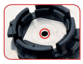
Before reinstalling the ball, check that the pipe is not blocked by blowing into it, from the opposite side to the picture above.
