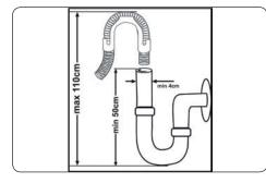
Connect water drain hose directly to water drain hole or to the sink outlet spigot. This connection should be minimum 50cm and maximum 110cm from floor plane.
