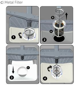
To remove and clean the filter combination, turn it counter clockwise and remove it by lifting it upwards (1).Pull the coarse filter out of the micro filter (2).Then pull and remove the metal filter (3).Rinse the filter with lots of water until it is free of residue. Reassemble the filters. Replace the filter insert, and rotate it clockwise (4).
