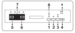
You can press the On/Off button (4) to switch on the product. On/Off lights will be on so long as the machine is on. Press the program button (5) to set the suitable program.
