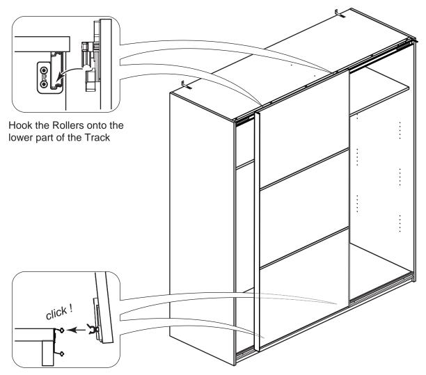
Line up the Bottom Guides with the top part of the Track and push the Door in until it clicks into place
