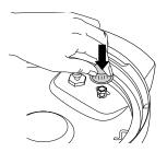
**NOTE:** Prior to each use, make sure the silicone ring is well seated in the silicone ring rack and the anti-clog cap is mounted properly on the pressure release valve.
