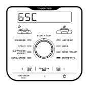
**3** Press TIME, then turn the dial to adjust the cook time in 15-minute increments up to 12 hours.
