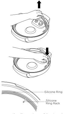
To remove the silicone ring, pull it outward, section by section, from the silicone ring rack. The ring can be installed with either side facing up. To reinstall, press it down into the rack section by section.
