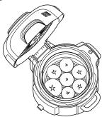
2 Press FUNCTION, then turn the START/STOP dial to select DEHYDRATE. The default temperature setting will display. Press TEMP, then turn the dial to choose a temperature between 25°C and 90°C.
