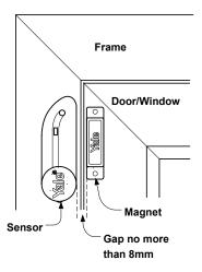
1 Find a location where the door/window contact is to be mounted. It should be mounted between the door/window frame and the door/window as shown at the top of the opening. The magnet is to go on the door/window while the sensor is to be placed on the frame. The gap between the magnet and sensor should be no more than 8mm when closed. Windows can be protected in a similar way to doors. Make sure the tamper switch spring is fully depressed.
