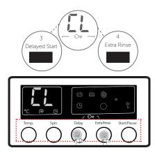
"CL" symbol will flash on the electronic display when activated.
