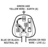
The BLUE wire must be connected to the terminal marked with the letter N p
