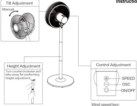
short press the key to adjust the wind speed, long press the key for 2 seconds to set the timer.
