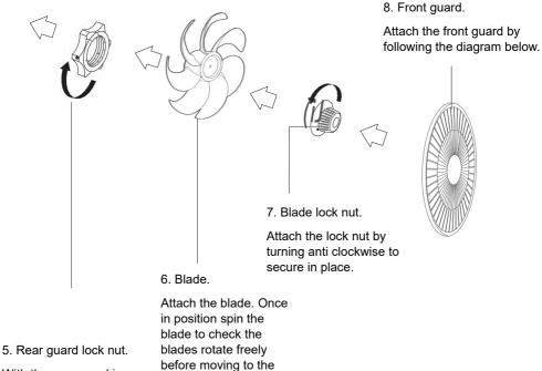
With the rear guard in position, screw the lock nut clockwise to secure.
