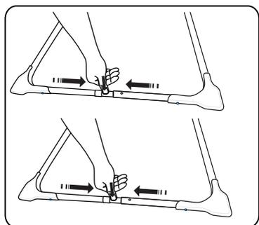
5.1 Insert the front leg with plastic part into another front leg , fix it by a screw.
