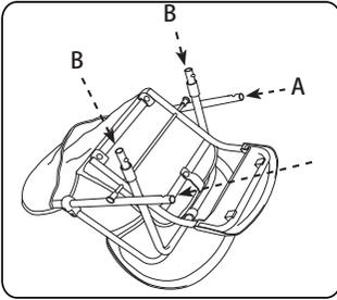
6.1 The front and rear legs have a different width. Please be aware that the rear leg is narrower at the top, than the front leg.
