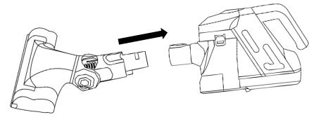
2. To use the floor head with the extension tube, place the extension tube onto the nozzle of the handheld unit, ensuring that the pins are aligned and click in to place.
