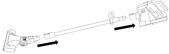
To remove the floor head, press the release button on the extension tube and pull away the floor head.
