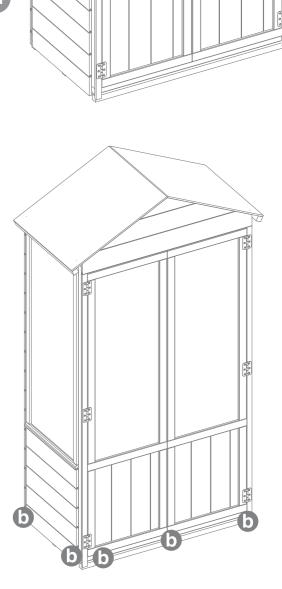
Fix the bottom shelf inbetween the window sides (inside the building) using 6x30mm screws.
