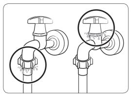
**3.** Slowly open the water tap and check if there are any leaks around the connection areas. If there are water leaks, repeat step 1 and 2.
