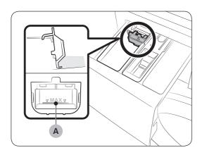
First insert the provided liquid detergent guide in the III main-wash compartment. Then, apply liquid detergent to the guide below the marked max line (A).
