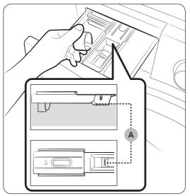
3. Apply fabric softener to the **softener** compartment. Do not exceed the max line (A). Softener is dispensed into the wash during the final rinse.
