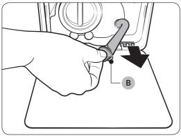
**3.** Put an empty, spacious container around the cover, and stretch the emergency drain tube to the container while holding the **tube cap (B)**.
