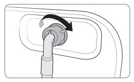
2. Connect the other end of the water hose to the inlet valve on the back of the washing machine, and then turn it to the right to tighten.
