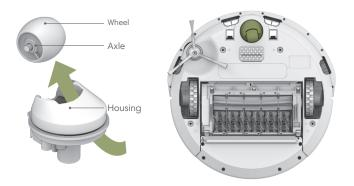
Important: A front wheel clogged with hair and debris could result in floor damage.
