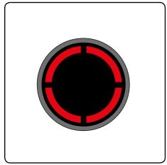
If the brush bar jams during use, the AirRam will stop and the LEDs will appear red. You will need to remove and clean the brush bar (see page 11).
