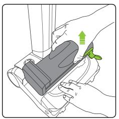
Holding onto the AirRam with one hand, pull the bin handle and lift the bin out of the AirRam.
