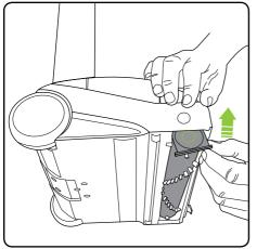
Re-insert the brush bar, starting by locating the end furthest away from the button. Then push the brush bar into the AirRam until it clicks into place.
