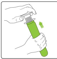
Slide the filter onto the inner shroud.
