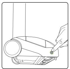
Rest the AirRam on its side and locate the brush bar button on the right hand side. Press the button inwards and then pull the brush bar towards the bottom of the AirRam.
