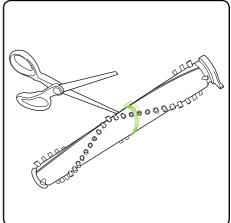
To remove hair from the brush bar, run an open pair of scissors down the groove to cut the hair, then pull it out.
