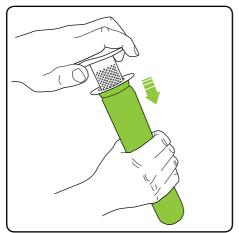
Remove the filter from the inner shroud, by twisting and pulling.
