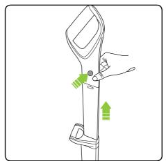
To extend the upper handle, hold down the button on the left hand side and pull it up. It will click into place.
