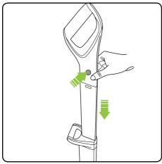
To stow the upper handle, simply press the button on the left hand side and push the handle down.
