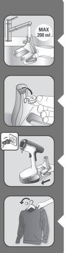
Fill the water tank with a maximum of 200 ml of untreated tap water.
