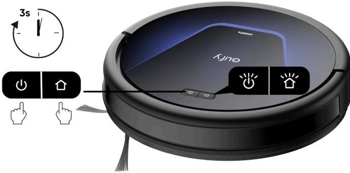
You will hear a voice prompt when the Wi-Fi connection has been reset, and the LED indicators on RoboVac will quickly flash white. Now you can follow the in-app instructions to reset the Wi-Fi connection.
