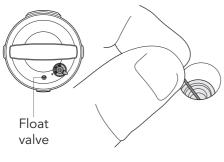
Cleaning the float valve: Clean the float valve using a pin to ensure there is no debris trapped inside or around it.
