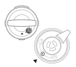
Turn the pressure release valve to the CLOSED position.
