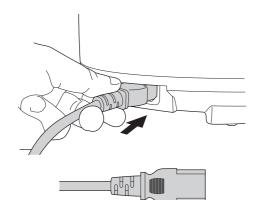
Slot the end of the power cord into the socket on the rear of the pressure cooker as shown in the diagram.
