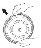
**Removing the gasket:** Pull the rubber gasket from the sides of the inner lid.
