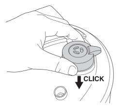
Lower the lid and slot the pressure valve into the large recess on the top of the pressure cookers lid.
