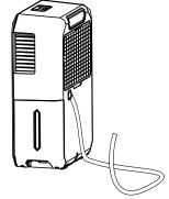
Do not block water flow by a retortion.
