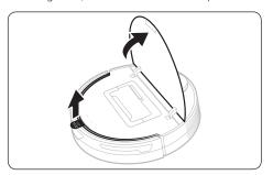
1 Open the upper cover of the Jet Bot and remove the white gasket.
