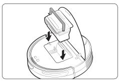
6 Attach the filter to the Dustbin and insert the Dustbin into the Jet Bot. When inserting the Dustbin, grasp the handle and put the Dustbin into both grooves.
