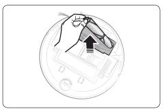
3 Lift up the left side of the brush first and then pull the brush from the groove on the right.
