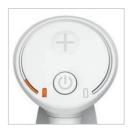
When less than 20% charge is remaining the indicator light will flash indicating the battery is running low.
