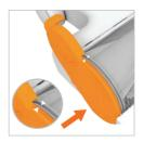
Line up the arrows and push the brushbar cover flush to the floorhead.
