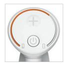
The battery level indicator will illuminate white to show the remaining runtime.
