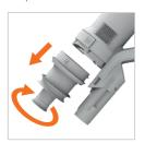
Twist and turn the separator to remove it from the handheld.
