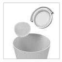
Tap the sponge filter and the frame over a bin to remove any dirt and debris.
