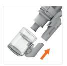
Line up the dirt release grip with the handheld and slide the dirt container into place. The dirt bin will click when correctly fitted.
