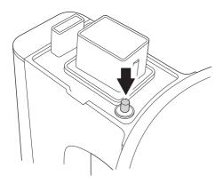
**IMPORTANT**: If when you press the saute button it does not work, the automatic shut off switch on the top of the handle may have become stuck.
