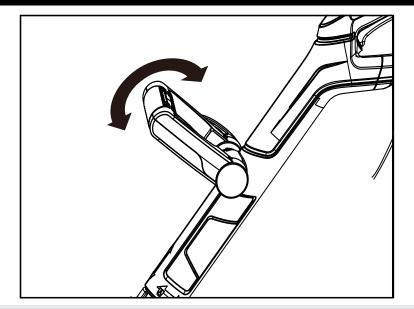
The front handle can be set to various positions. Set the handle in such a manner that the trimmer head is slightly tilting forwards when in the working position.
