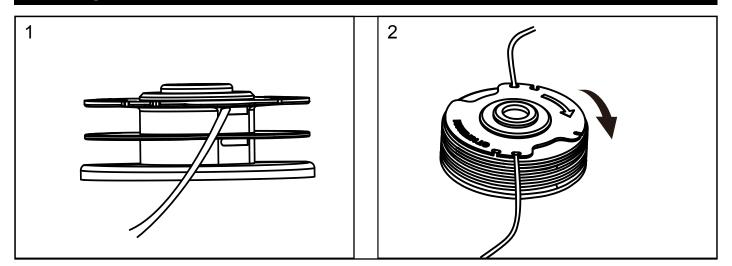
**NOTE:** Self-winding is not recommended. If the line is not wound properly it can cause the trimmer feed system to malfunction. For this reason, users are strongly urged to purchase the pre-wound spool.
