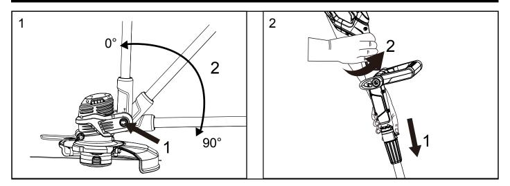
The trimmer head angle is adjusted by pressing the head adjustment button and moving the trimmer head to the desired angle. There are 7 snap-in positions between 0° and 90° See figure 1.
