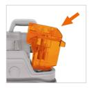
Refit the dirty water tank onto the machine so it clicks into place.
