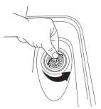
4 Clean removed burr grinder with brush.
