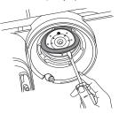
**4** Insert shower screen back into group head and secure in position with screw.
