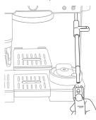
**3** For a deeper clean, use the wrench in the middle of the cleaning brush to remove the steam wand tip.
