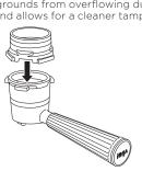
2 With the funnel on top of the portafilter, insert into the grinding cradle. Make sure it is level and fits securely. Once portafilter is installed in grinding cradle, it will be weighed. To ensure accurate weight, let go of portafilter.
