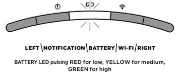
If your robot is low on battery power, the left LED light will pulse RED. Manually place the robot on the base to begin charging. When the robot is charging, the battery indicator light will pulse, based on the current battery charge level: RED for low, YELLOW for medium, GREEN for high.
