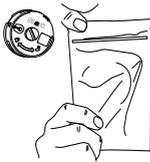
4. Align the yellow arrow on the side of the cartridge with the yellow arrow on the side of the dial cover, then insert the cartridge into the dial. Rotate the cartridge clockwise to lock it in place.
