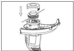
**NOTE:** Before replacing the spool, make sure the mains plug is disconnected from the unit.
