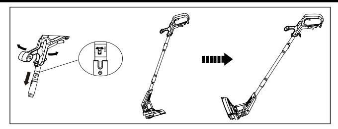
• When trimming near edges and walls, push the shaft forward, turn the handle to 180°.
