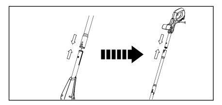
• Insert the upper and lower shaft handles securely into the middle handle shaft and ensure they are fully engaged and locked into position.
