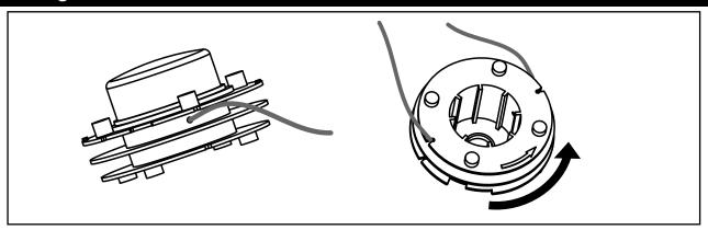
**NOTE:** Self-winding is not recommended. If the line is not wound properly it can cause the trimmer feed system to malfunction. For this reason, users are strongly urged to purchase the pre-wound spool.
