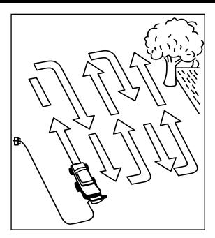
Place the mains lead in loops on the ground near the wall socket. Mow away from
