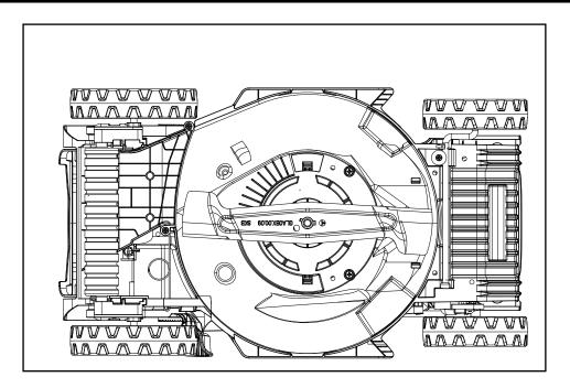
If the blade is blunt, it can be sharpened in a specialised workshop. If the blade is damaged or showing signs of imbalance, it must be replaced.
