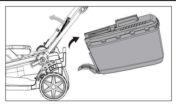
To remove the grass collector, raise the deflector guard with one hand and remove the grass collector holding its handle with your other hand. To maintain safety, the deflector guard automatically closes to the rear discharge position when you remove the grass collector.
