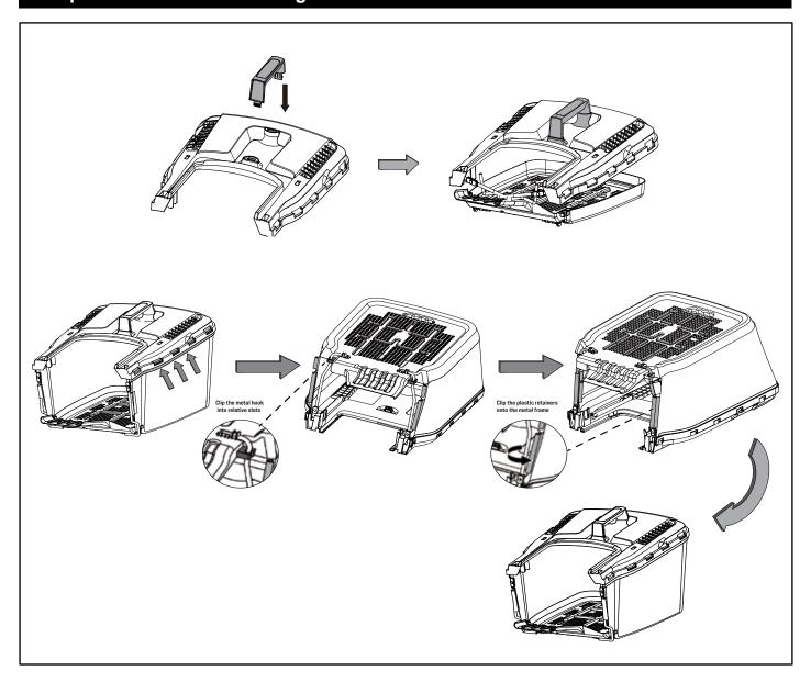
• Insert the handle into the slots on the top of the grass collection bag. Clip the plastic retainers found on both sides of the cloth bag onto the metal frame of the plastic upper. Fully insert the rods of the metal frame into the slots on either side of the plastic base. Ensure the side clamping sleeves are properly fixed onto the frame.
