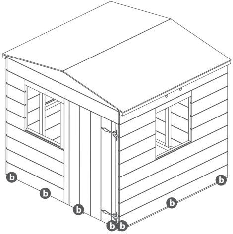
Cut the felt into 2 sheets and lay onto the roof as shown in the diagram ensuring there is a 50mm overhang around the sides.
