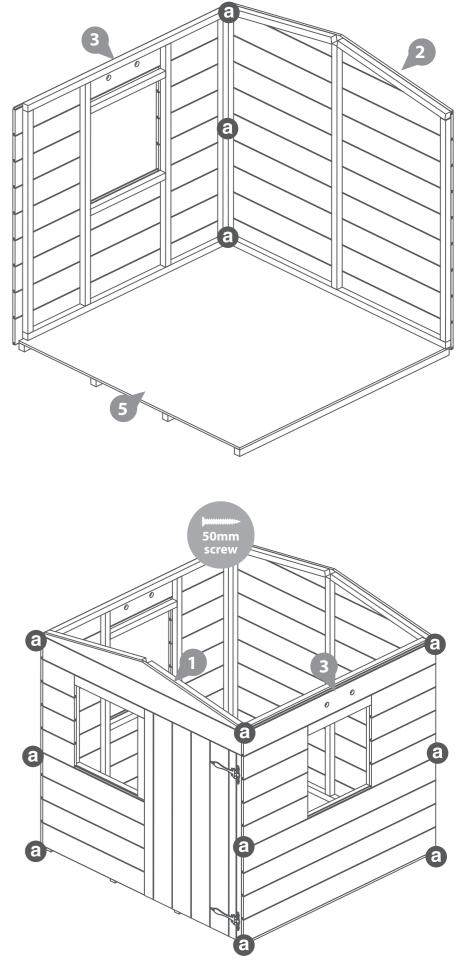
Position the panels so there are equal gaps between the floor and cladding
