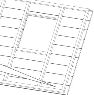
Lay the door gable face up on a flat surface, place the door within the door aperture. Position the door so that you have a equal gap either side of the door to the gable.
