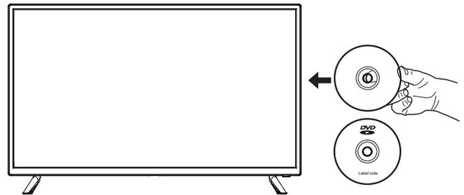
**Note:** Only use fixed outer diameter 120mm disc, use other size disc may cause card disc!
