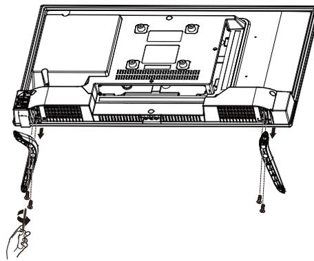
4. Use the four screws (M4\*6mm, not included) to fix the TV onto a wall mounting bracket (not included) via the four VESA standard holes on the back of the television.
