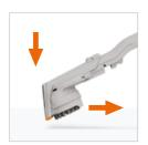
Tilt the nozzle forward so the nozzle is in contact with the surface. Pull back to recover the water and solution.
