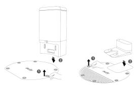
2 Remove the water tank from the main unit. Open the water inlet cover to fill the water, then close the cover.
