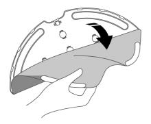
**5** Wet the mopping cloth and wring out excess water. Slide the mopping cloth all the way back onto the slot of the mopping module and stick it firmly.
