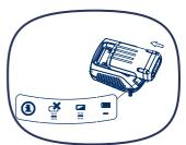
You can read the battery pack's remaining charge by using the chart.
