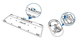
Connect the wireless dongle for keyboard and mouse to a USB port to automatically pair both devices to your ASUS All-in-One PC.
